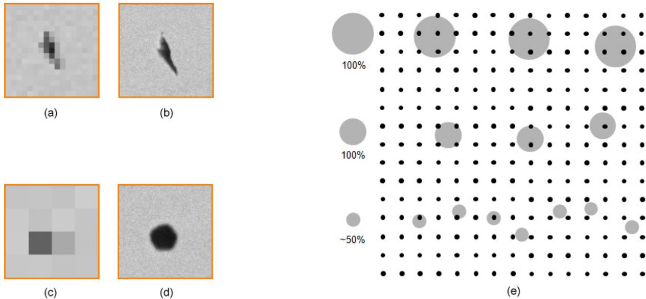
Figure 4 – Detection of Inclusions in CCSEM Search Mode: (a) Multi-Pixel Inclusion in Search Field; (b) Same Inclusion in Microimage; (c) Single-Pixel Inclusion in Search Field; (d) Same Inclusion in Microimage; (e) Simplified Schematic of Detection Probability
