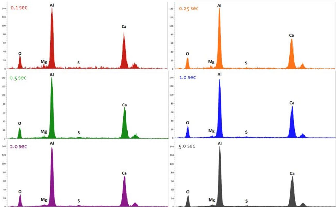
Figure 6 - - EDS Spectra at 45Kcps of Single Spectra at Various Collection Times. Horizontal Scale is 0-5 keV
