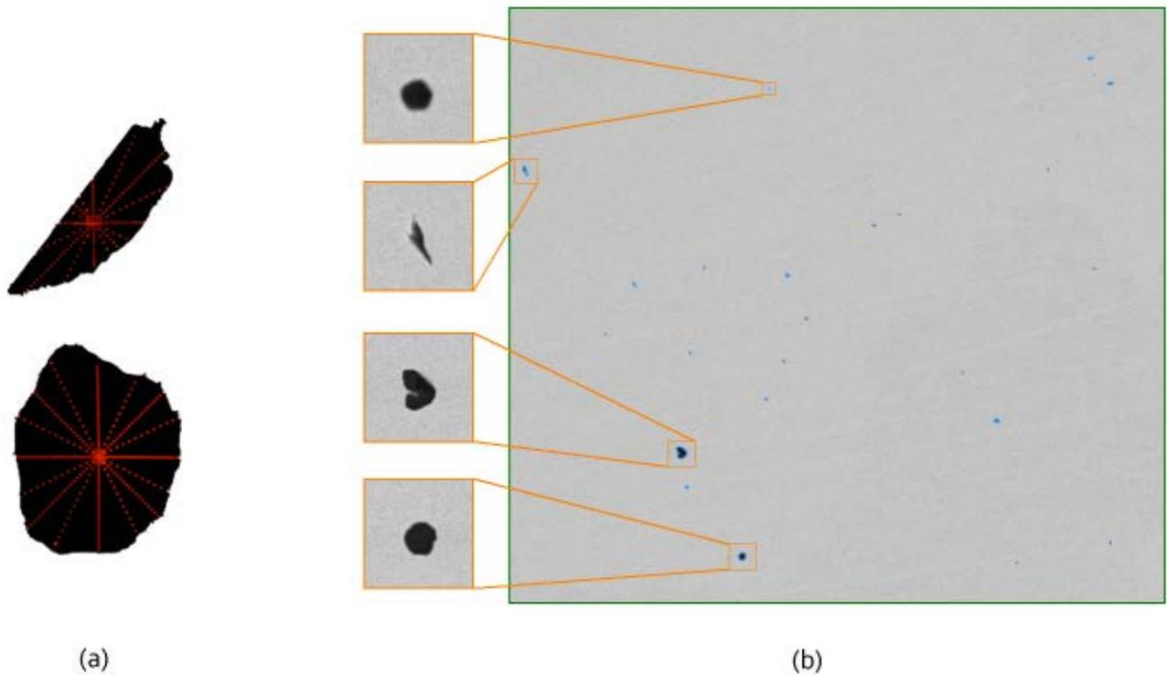
Figure 3 - (a) Rotated-chord measurement technique; (b) Microimage measurement technique
