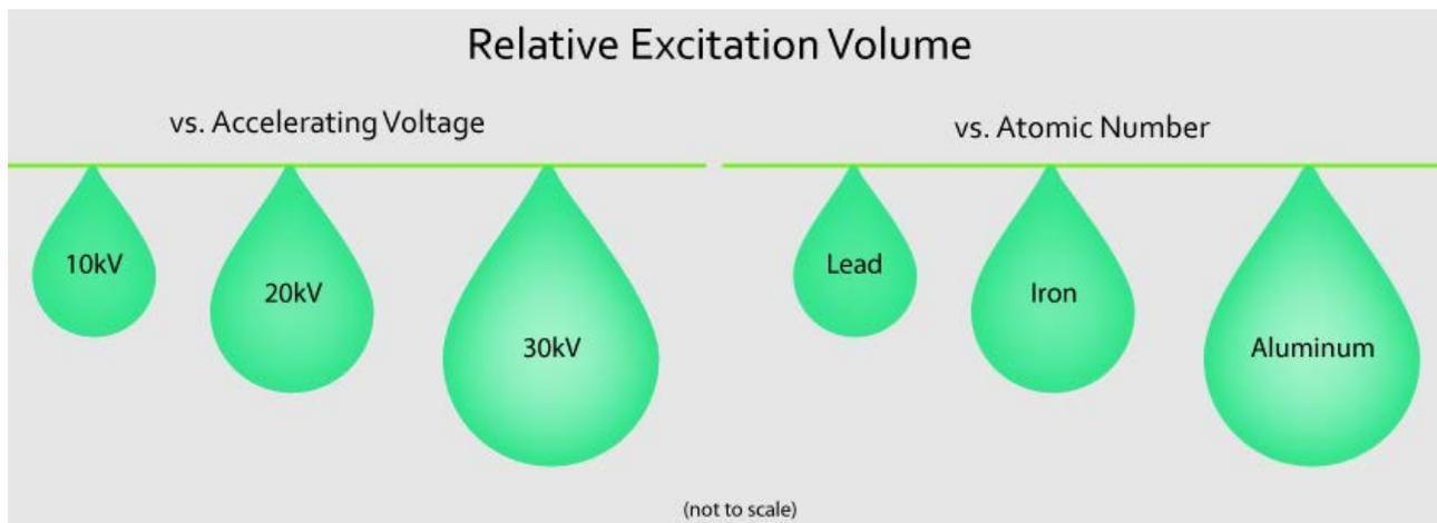
Figure 8 - Comparative Effect of Accelerating Voltage (left) and Atomic Number (right) on Excitation Volume
