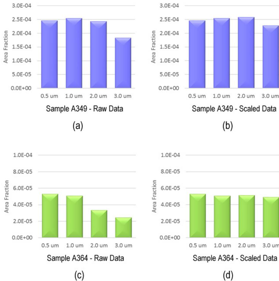
Figure 5. Area Fraction of Inclusions Using Different Pixel Densities.
