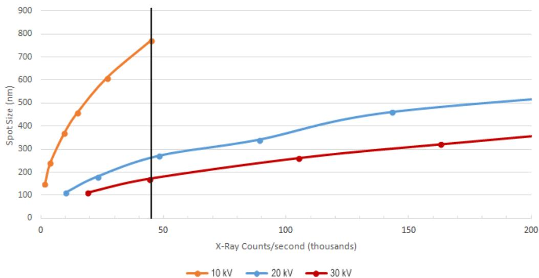
Figure 9 - Spot Size Versus Count Rate for Various Accelerating Voltages. Vertical Line Indicates 45kcps
